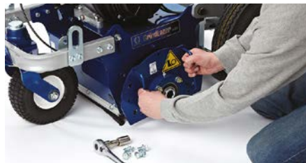
2. Remove bolts and door
