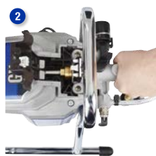
Remove pump section
