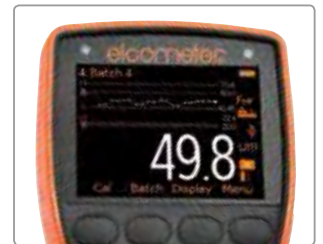
The Run Chart displays each individual reading allowing the user to identify any significant trends
