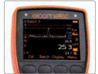
The Run Chart displays the average thickness as well as the highest and lowest readings for each scan
