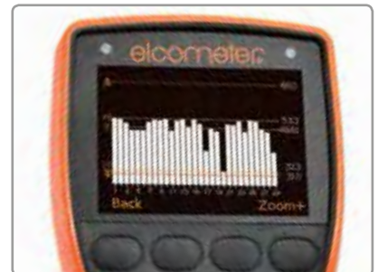
Individual batch readings can be reviewed numerically or graphically
